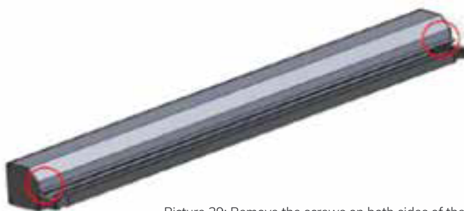
Picture 29: Remove the screws on both sides of the smart.
