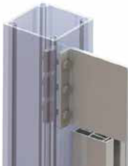
Drawing 24: Screwing the angle bracket to the post.
